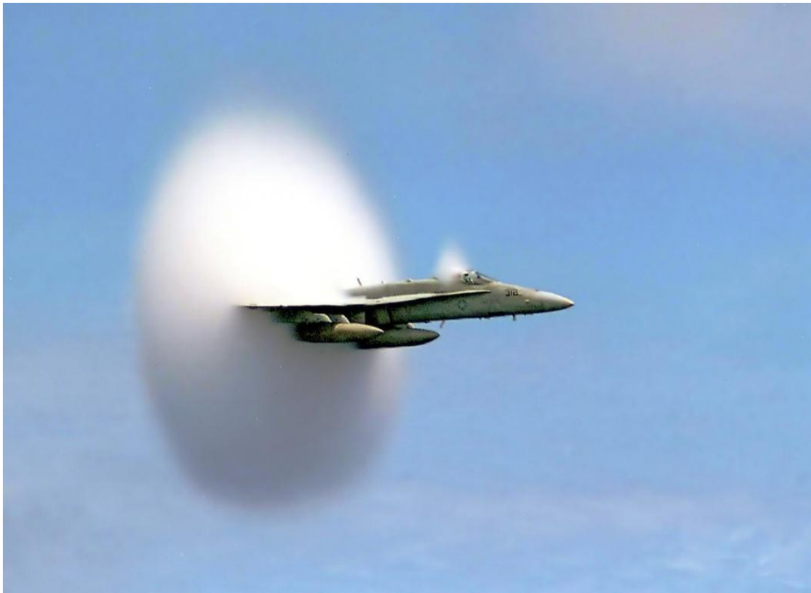
A rare picture of an F-18 Hornet displaying localized condensation near the speed of sound. Courtesy Wikipedia
